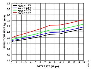
Figure 8. Supply Current (IDD1) vs. Data Rate
