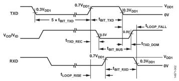
Figure 2. Transceiver Timing Diagram
