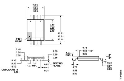
Figure 29. 8-Lead Standard Small Outline Package, with Increased Creepage [SOIC\_IC] Wide Body (RI-8-1)Dimensions shown in millimeters
