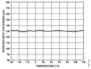
Figure 10. Receiver Input Hysteresis vs. Temperature
