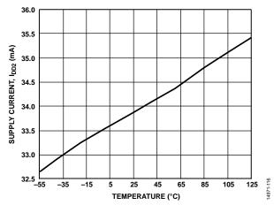
Figure 18. Supply Current (IDD2) vs. Temperature
