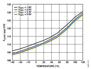
Figure 13. t<sub>LOOP\_RISE</sub> vs. Temperature
