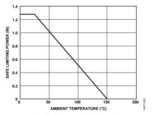
Figure 5. ADM3050EBRIZ Thermal Derating Curve, Dependence of Safety Limiting Values with Ambient Temperature per DIN V VDE V 0884-10 (See the Thermal Resistance Section for Additional Information)
