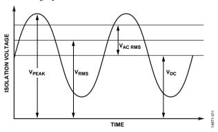
Figure 27. Critical Voltage Example
