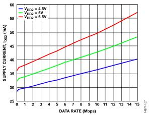
Figure 9. Supply Current (IDD2) vs. Data Rate
