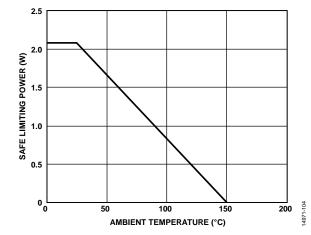
Figure 4. ADM3050EBRWZ Thermal Derating Curve, Dependence of Safety Limiting Values with Ambient Temperature per DIN V VDE V 0884-10 (See the Thermal Resistance Section for Additional Information)
