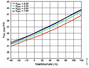
Figure 11. t<sub>TXD\_DOM</sub> vs. Temperature
