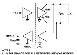
Figure 22. Switching Characteristics Measurements
