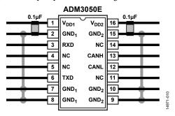
Figure 25. Recommended 16-Lead SOIC\_W PCB Layout
