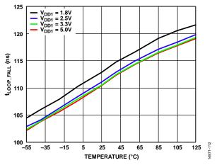
Figure 14.  $t_{\text{LOOP\_FALL}}$  vs. Temperature
