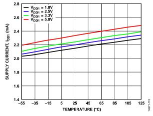
Figure 17. Supply Current (IDD1) vs. Temperature
