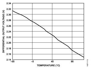
Figure 15. Differential Output Voltage vs. Temperature,  $R_L = 60 \Omega$
