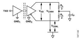
Figure 20. Driver Voltage Measurement
