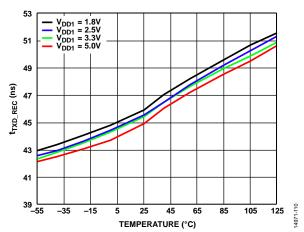
Figure 12. t<sub>TXD\_REC</sub> vs. Temperature
