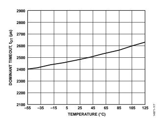
Figure 19. Dominant Timeout (t<sub>DT</sub>) vs. Temperature
