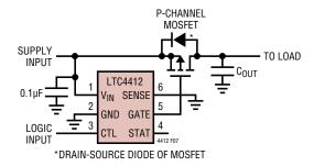
Figure 7. Logic Controlled High Side Power Switch
