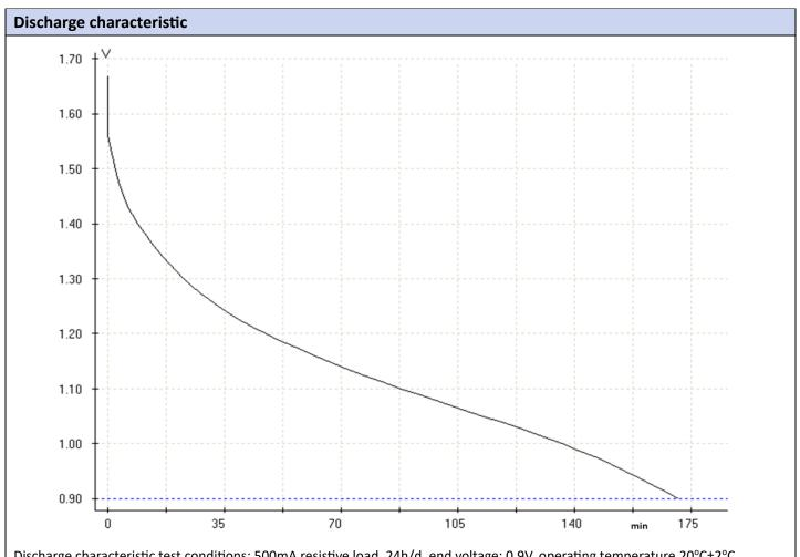
Discharge characteristic test conditions: 500mA resistive load, 24h/d, end voltage: 0.9V, operating temperature 20°C±2°C
