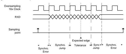
Figure 24-48. Bit Resynchronization
