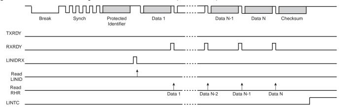
Figure 24-39. Slave Node Configuration, LINMR.NACT is 0x2 (IGNORE)
