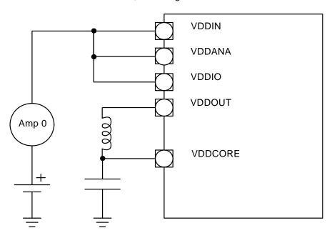
Figure 42-2. Measurement Schematic, Switching Mode
