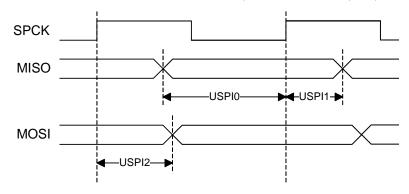
**Figure 42-8.** USART in SPI Master Mode with (CPOL= 0 and CPHA= 1) or (CPOL= 1 and CPHA= 0)
