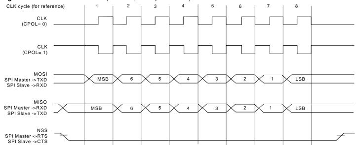
Figure 24-44. SPI Transfer Format (CPHA=0, 8 bits per transfer)
