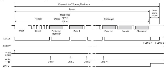
Figure 24-35. Master Node Configuration, LINMR.NACT is 0x1 (SUBSCRIBE)
