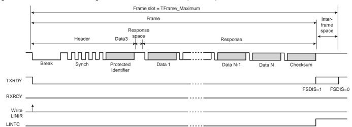
Figure 24-36. Master Node Configuration, LINMR.NACT is 0x2 (IGNORE)
