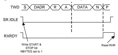
Figure 27-9. Master Read with Multiple Data Bytes
