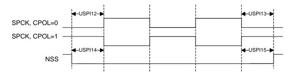
Table 42-58. USART0 in SPI mode Timing, Slave Mode<sup>(1)</sup>
