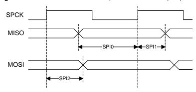
Figure 42-13. SPI Master Mode with (CPOL= 0 and NCPHA= 1) or (CPOL= 1 and NCPHA= 0)
