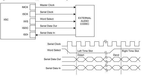
Figure 29-6. Codec Application Block Diagram
