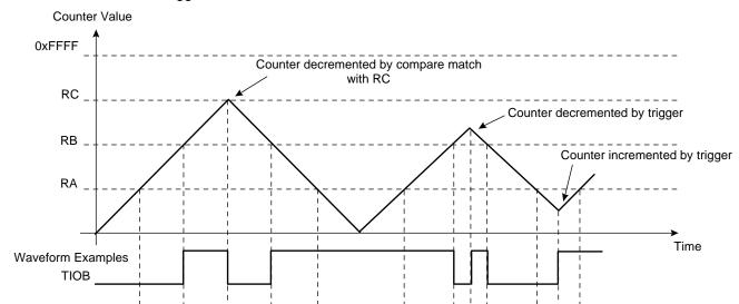
Figure 30-12. WAVSEL = 3 With Trigger
