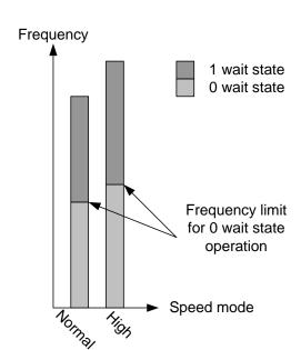
Figure 14-3. High Speed Mode
