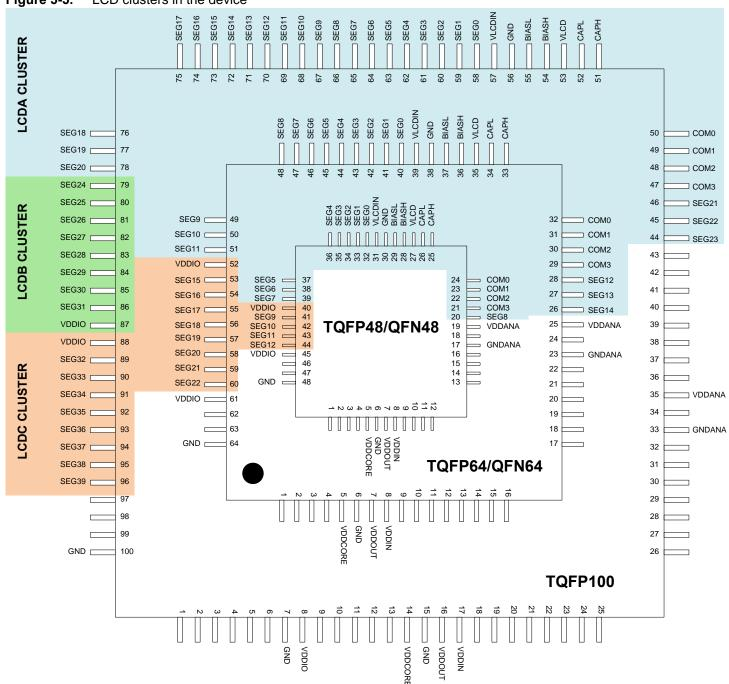
Figure 5-5. LCD clusters in the device
