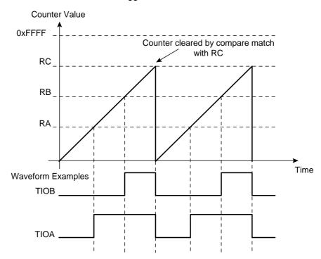
Figure 30-7. WAVSEL = 2 Without Trigger
