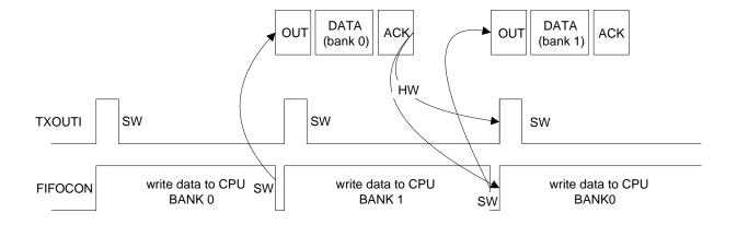
DATA DATA OUT **ACK** OUT **ACK** (bank 0) (bank 1) HW **TXOUTI** SW SW SW write data to CPU write data to CPU write data to CPU **FIFOCON** SW SW BANK 0 BANK 1 BANK<sub>0</sub>
