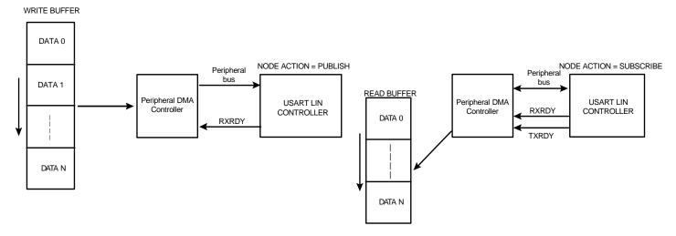
Figure 24-41. Master Node with Peripheral DMA Controller (LINMR.PDCM=1)
