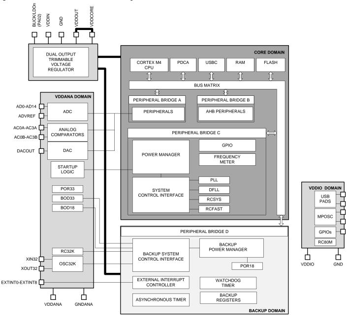
Figure 5-2. ATSAM4LC Power Domain Diagram
