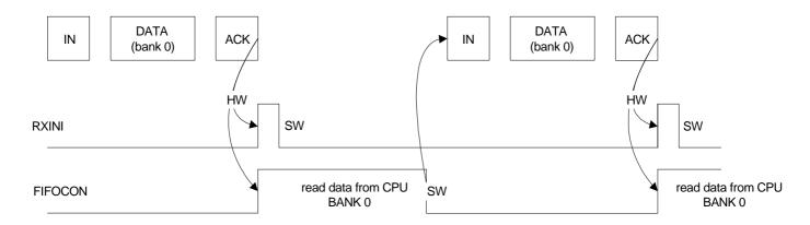
Figure 17-18. Example of an IN pipe with two data banks
