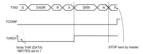
Figure 28-8. Slave Transmitter with Multiple Data Bytes
