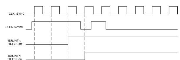
Figure 21-2. Timing Diagram, Synchronous Interrupts, High Level or Rising Edge
