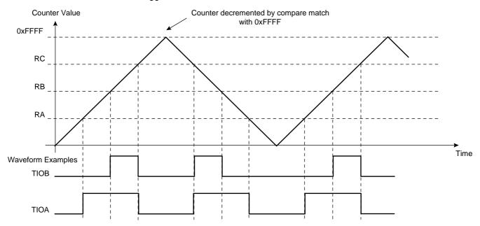
Figure 30-10. WAVSEL = 1 With Trigger
