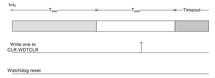
Figure 20-5. Window Mode WDT Timing Diagram, clearing within T<sub>than</sub>, resulting in watchdog reset.
