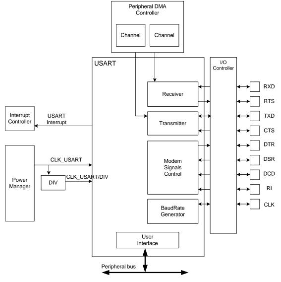
Figure 24-2. USART Block Diagram
