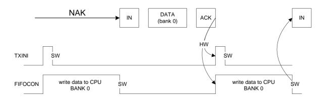
Figure 17-10. Example of an IN endpoint with two data banks
