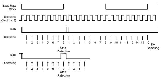
Figure 24-6. Asynchronous Mode Character Reception
