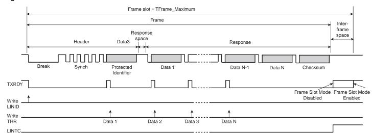
Figure 24-33. Frame Slot Mode with Automatic Checksum
