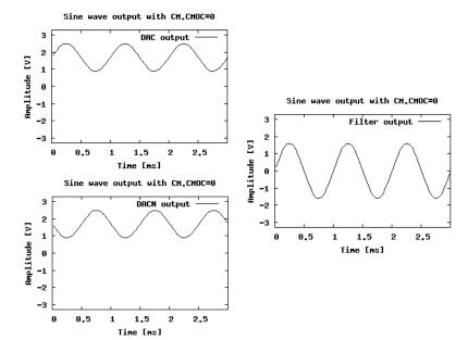
Figure 32-2. Output signals with CMOC=0
