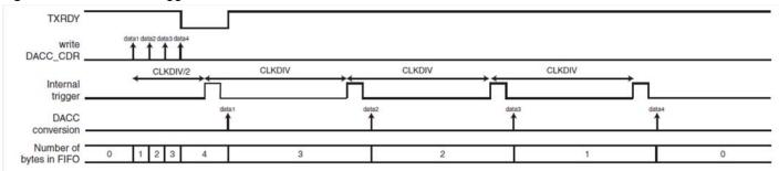
Figure 33-3. External Trigger
