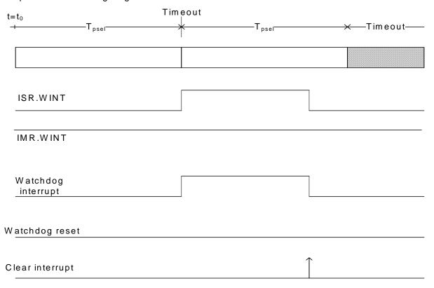
Figure 20-7. Interrupt Mode WDT Timing Diagram, not clearing the interrupt.
