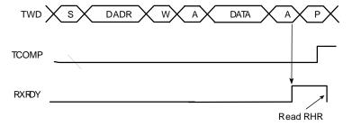
Figure 28-11. Slave Receiver with Multiple Data Bytes
