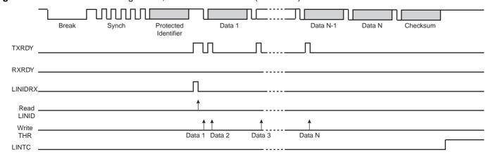
Figure 24-38. Slave Node Configuration, LINMR.NACT is 0x1 (SUBSCRIBE)
