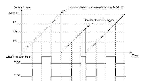
Figure 30-6. WAVSEL= 0 With Trigger
