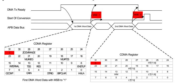
Figure 38-3. Two DMA Tx transfers: With Window Mode Configuration
