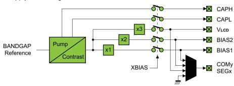
Figure 39-14. Internal and External Bias Generation
