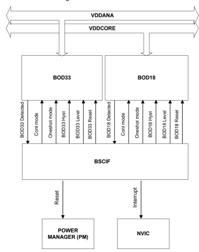
Figure 12-2. BOD18/33 Block Diagram
