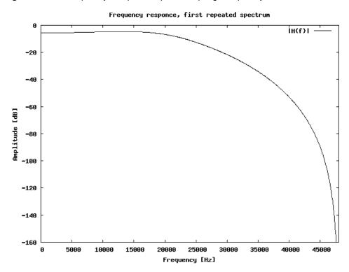
Figure 32-5. Frequency Response up to Sampling Frequency
