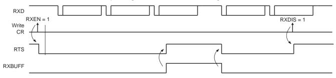
Figure 24-20. Transmitter Behavior when Operating with Hardware Handshaking
