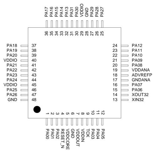
Figure 3-10. ATSAM4LS TQFP48/QFN48 Pinout
