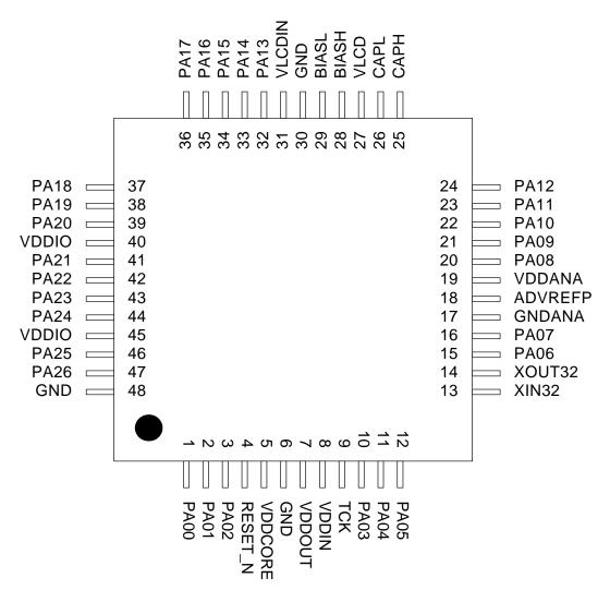
Figure 3-5. ATSAM4LC TQFP48/QFN48 Pinout
