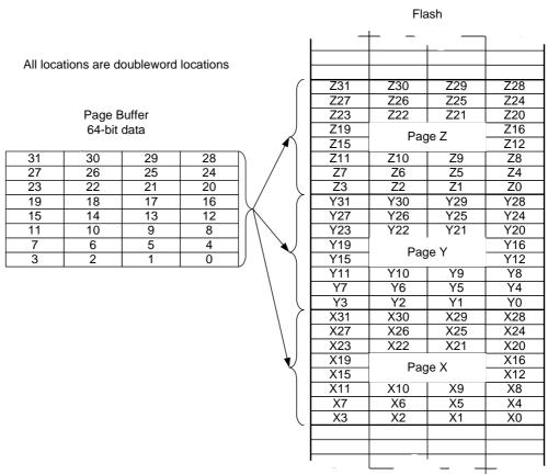
Figure 14-4. Mapping from Page Buffer to Flash
