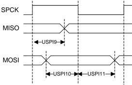
Figure 42-11. USART in SPI Slave Mode, NPCS Timing
