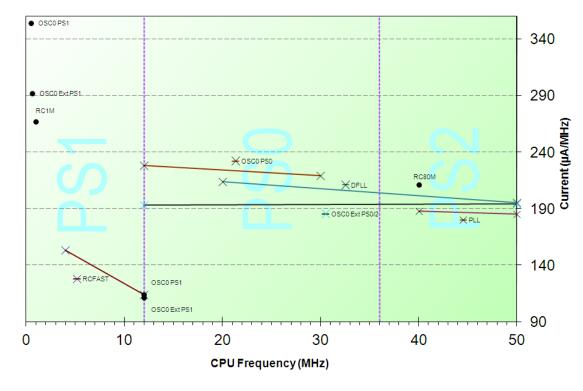
Figure 42-1. Typical Power Consumption running Coremark (from above table)
