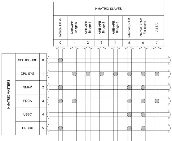
Figure 15-1. HMatrix Master / Slave Connections
