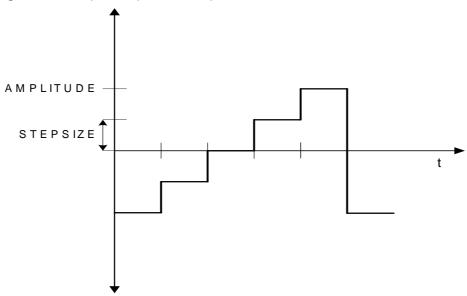
Figure 13-6. Spread Spectrum Sequence added to FINE Value
