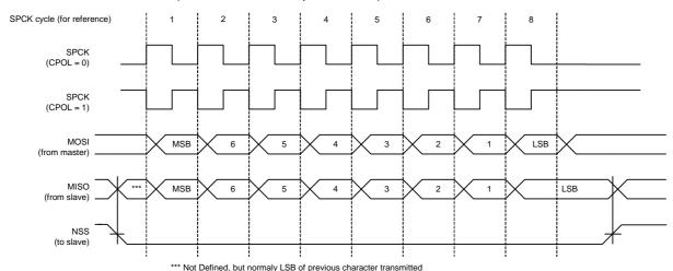
Figure 26-4. SPI Transfer Format (NCPHA = 0, 8 bits per transfer)
