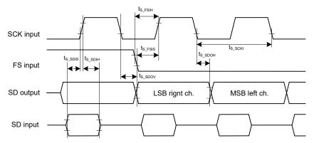
Figure 37-26. I2S Timing PDM2 Mode
