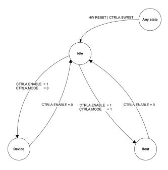
After a hardware reset, the USB is in the idle state. In this state:
