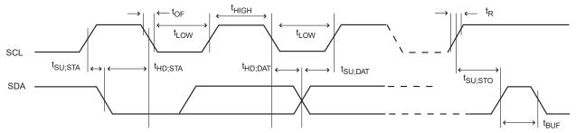
Table 37-68. I<sup>2</sup>C Interface Timing (Device Variant A)
