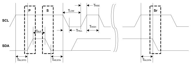
The following parameters are timed using the SCL low time period T<sub>LOW</sub>. This comes from the Host Baud Rate Low bit group in the Baud Rate register (BAUD.BAUDLOW). When BAUD.BAUDLOW=0, or the Host Baud Rate bit group in the Baud Rate register (BAUD.BAUD) determines it.
