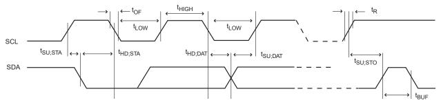
Table 41-55. I<sup>2</sup>C Interface Timing (Device Variant A)
