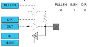
Figure 23-5. I/O Configuration - Input with Pull
