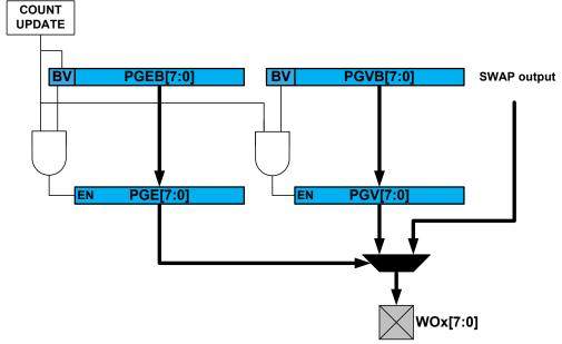
As with other double-buffered timer/counter registers, the register update is synchronized to the UPDATE condition set by the timer/counter waveform generation operation. If synchronization is not required by the application, the software can simply access directly the PATT.PGE, PATT.PGV bits registers.
