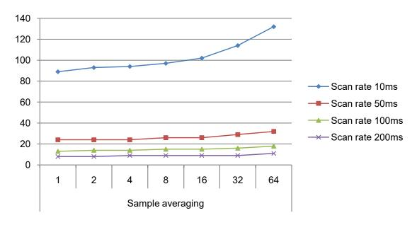
Figure 37-8. Power Consumption [μA] 1 sensor, noise countermeasures Enabled, f=48MHz, Vcc=3.3V
