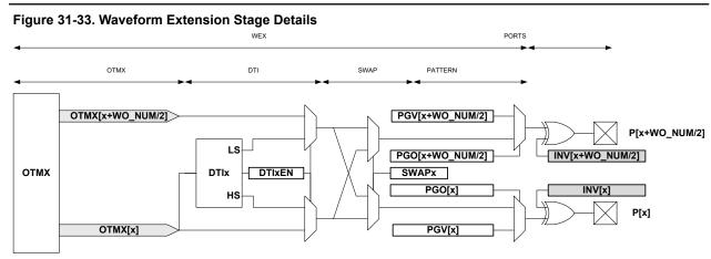
The output matrix (OTMX) unit distributes compare channels, according to the selectable configurations in Table 31-4.
