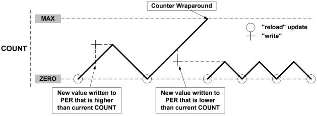
When double buffering is used, the buffer can be written at any time and the counter will still maintain correct operation. The period register is always updated on the update condition, as shown in Figure 31-13. This prevents wraparound and the generation of odd waveforms.
