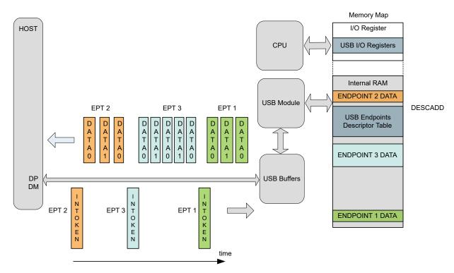
When an IN token is detected, and if the device address of the token packet does not match DADD.DADD, the packet is discarded and the USB module returns to idle and waits for the next token packet.
