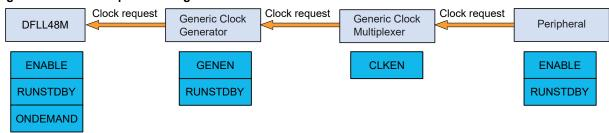
All clock sources in the system can be run in an on-demand mode: the clock source is in a stopped state unless a peripheral is requesting the clock source. Clock requests propagate from the peripheral, via the GCLK, to the clock source. If one or more peripheral is using a clock source, the clock source will be started/kept running. As soon as the clock source is no longer needed and no peripheral has an active request, the clock source will be stopped until requested again.
