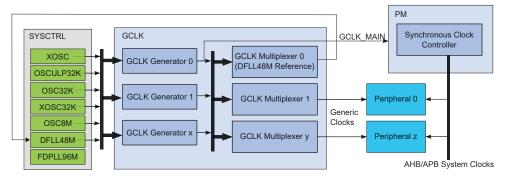
The clock system on the SAM D21 consists of:
