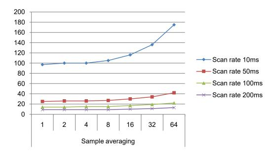
Figure 41-9. Power Consumption [μA] 10 sensors, noise countermeasures disabled, f=48MHz, Vcc=3.3V
