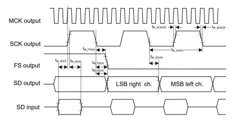
Figure 37-25. I<sup>2</sup>S Timing Client Mode
