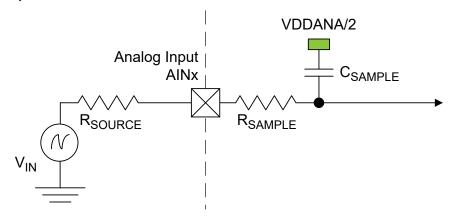
To achieve n bits of accuracy, the C<sub>SAMPLE</sub> capacitor must be charged at least to a voltage of
