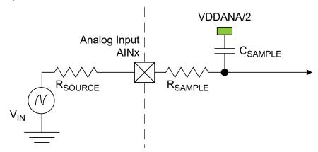
To achieve n bits of accuracy, the  $\mathcal{C}_{SAMPLE}$  capacitor must be charged at least to a voltage of
