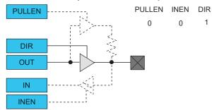
Figure 23-7. I/O Configuration - Totem-Pole Output with Enabled Input
