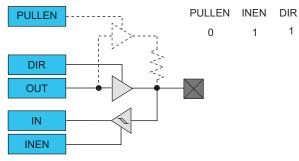
Figure 23-8. I/O Configuration - Output with Pull
