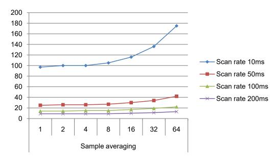
Figure 37-9. Power Consumption [μA] 10 sensors, noise countermeasures disabled, f=48MHz, Vcc=3.3V
