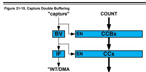
The TCC can detect capture overflow of the input capture channels: When a new capture event is detected while the Capture Buffer Valid flag (STATUS.CCBV) is still set, the new timestamp will not be stored and INTFLAG.ERR will be set.
