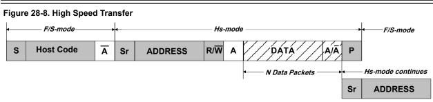
Transmitting in High-speed mode requires the I<sup>2</sup>C host to be configured in High-speed mode (CTRLA.SPEED=0x2) and the SCL Clock Stretch mode (CTRLA.SCLSM) bit set to '1'.
