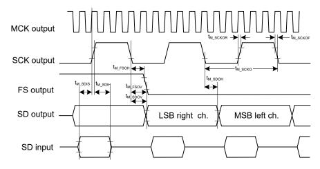
Figure 41-25. I<sup>2</sup>S Timing Client Mode
