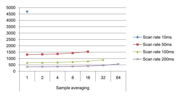
Figure 41-12. Power Consumption [μA] 100 sensors, noise countermeasures Enabled, f=48MHz, Vcc=3.3V
