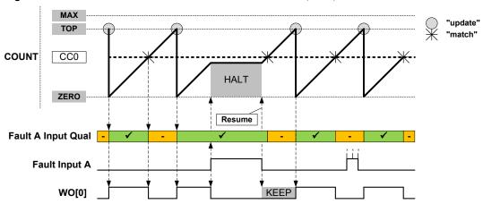
Software Halt Action This is configured by writing 0x2 to the Fault n Halt mode bits in the Recoverable Fault n configuration register (FCTRLn.HALT). Software halt action is similar to hardware halt action, but in order to restart the timer/counter, the corresponding fault condition must not be present anymore, and the corresponding FAULT n bit in the STATUS register must be cleared by software.
