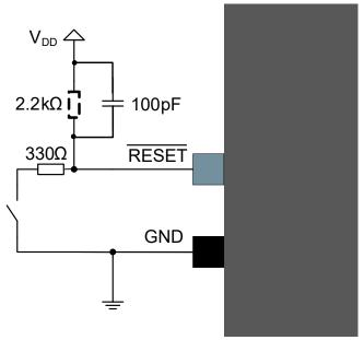
**Note:** This reset circuit is intended to improve EFT immunity, but does not filter low-frequency glitches, which makes it not suitable as an example for applications requiring debouncing on a reset button.
