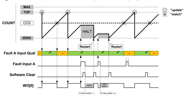
Figure 31-32. Waveform Generation with Software Halt, Fault Qualification, Keep and Restart Actions
