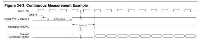
For low-power operation, comparisons can be performed during sleep modes without a clock. The comparator is enabled continuously, and changes of the comparator state are detected asynchronously. When a toggle occurs, the Power Manager will start CLK\_AC\_DIG to register the appropriate peripheral events and interrupts. The CLK AC DIG clock is then disabled again automatically, unless configured to wake up the system from sleep.
