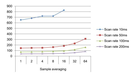
Figure 41-11. Power Consumption [μA] 100 sensors, noise countermeasures disabled, f=48MHz, Vcc=3.3V
