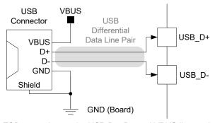
It is recommended to increase ESD protection on the USB D+, D-, and VBUS lines using dedicated transient suppressors. These protections should be located as close as possible to the USB connector to reduce the potential discharge path and reduce discharge propagation within the entire system.
