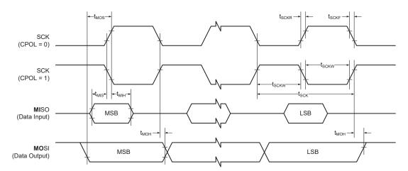
Figure 37-21. SPI Timing Requirements in Client Mode
