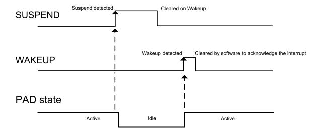
The Suspend Interrupt bit in the Device Interrupt Flag register (INTFLAG.SUSPEND) is set when a USB Suspend state has been detected on the USB bus. The USB pad is then automatically put in the Idle state. The detection of a non-idle state sets the Wake Up Interrupt bit (INTFLAG.WAKEUP) and wakes the USB pad.
