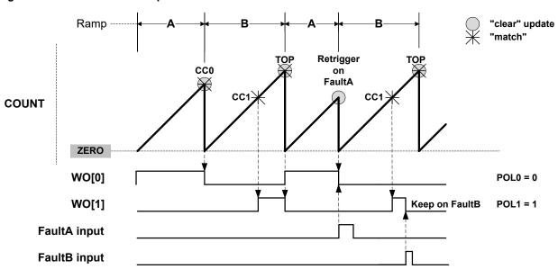
Figure 31-21. RAMP2 Critical Operation With 2 Channels
