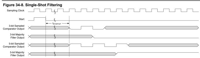
During sleep modes, filtering is supported only for single-shot measurements. Filtering must be disabled if continuous measurements will be done during sleep modes, or the resulting interrupt/event may be generated incorrectly.
