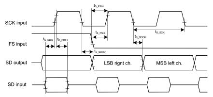
Figure 41-26. I<sup>2</sup>S Timing PDM2 Mode
