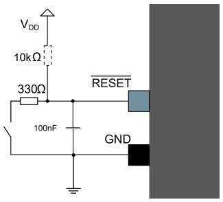
Figure 45-5. External Reset Circuit Schematic (EFT Immunity Enhancement)
