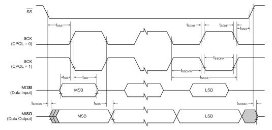
Table 37-67. SPI Timing Characteristics and Requirements<sup>(1)</sup>
