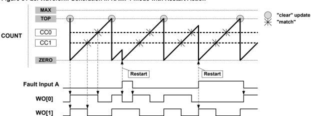
Figure 31-26. Waveform Generation in RAMP1 mode with Restart Action
