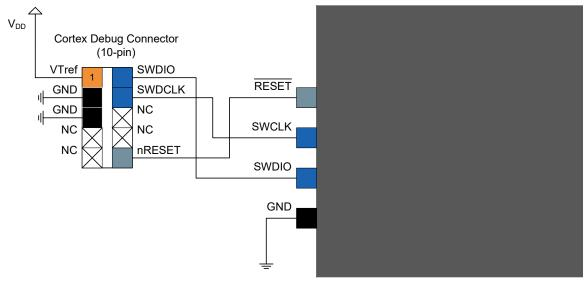
Table 45-9. Cortex Debug Connector (10-pin)
