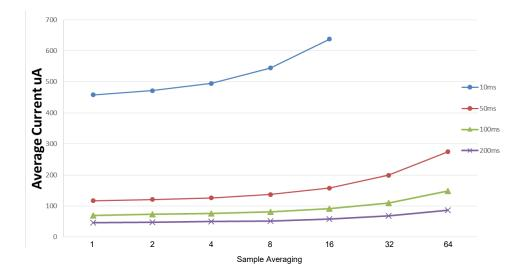
Figure 37-18. 100 Sensor / PTC\_GCLK = 4 MHz / FREQ\_MODE\_NONE
