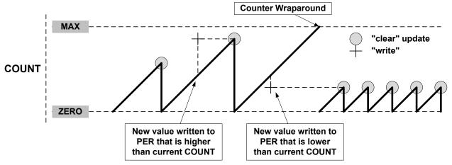
Figure 31-11. Unbuffered Single-Slope Down-Counting Operation
