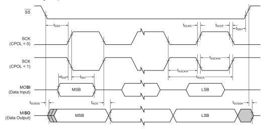
Table 41-54. SPI Timing Characteristics and Requirements<sup>(1)</sup>
