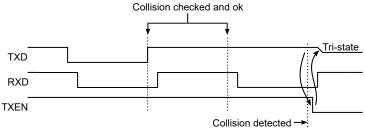
When a collision is detected, the USART follows this sequence:
