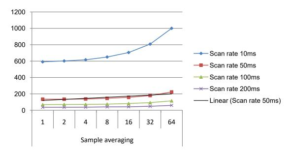
Figure 37-10. Power Consumption [μA] 10 sensors, noise countermeasures Enabled, f=48MHz, Vcc=3.3V
