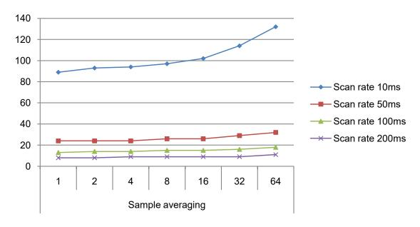
Figure 41-8. Power Consumption [μA] 1 sensor, noise countermeasures Enabled, f=48MHz, Vcc=3.3V
