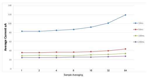
Figure 37-15. 1 Sensor / PTC\_GCLK = 2 MHz / FREQ\_MODE\_HOP
