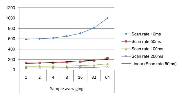
Figure 41-10. Power Consumption [μA] 10 sensors, noise countermeasures Enabled, f=48MHz, Vcc=3.3V
