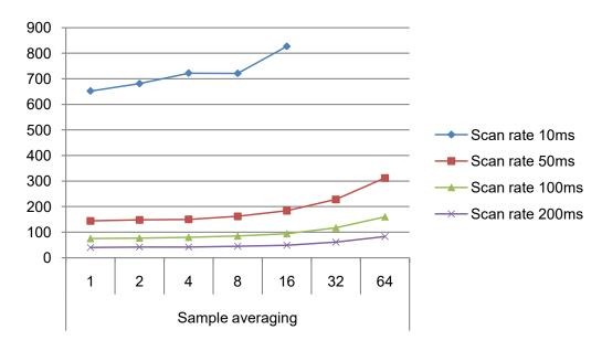
Figure 37-11. Power Consumption [μA] 100 sensors, noise countermeasures disabled, f=48MHz, Vcc=3.3V
