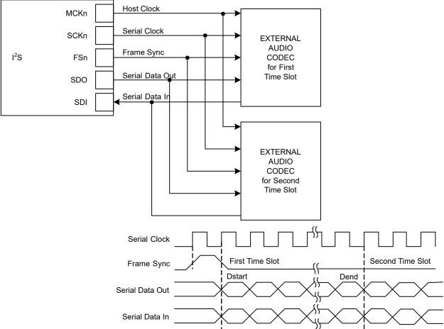
Figure 29-9. Codec Application Block Diagram
