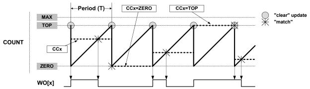
The following equation calculates the exact resolution for a single-slope PWM (R<sub>PWM\_SS</sub>) waveform:
