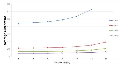
Figure 37-17. 10 Sensor / PTC\_GCLK = 2 MHz / FREQ\_MODE\_HOP
