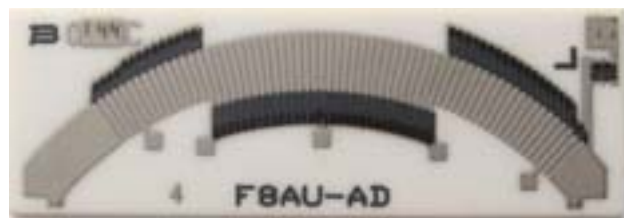
Figure 9: Single track design
