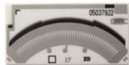
Figure 8: Dual track design
