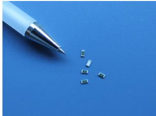
Following electronic product specifications apply to SMD fuses of the 123 series. The 123 series is a time-lag type subminiature fuse for over-current protection.
