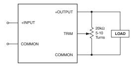
Figure 3. Trim Connections Using a Trimpot
