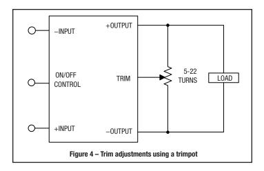
cause instability or oscillation. Keep external connections short to the Trim input. Use shielding if needed.
