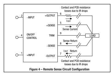
The remote Sense lines carry very little current. They are also capacitively coupled to the output lines and therefore are in the feedback control loop to regulate and stabilize the output. As such, they are not low impedance inputs and must be treated with care in PC board layouts. Sense lines on the PCB should run adjacent to DC signals, preferably Ground. In cables and discrete wiring, use twisted pair, shielded tubing or similar techniques.
