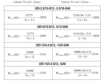
Where Vo = Desired output voltage. Adjustment accuracy is subject to resistor tolerances and factory-adjusted output accuracy. Mount trim resistor close to converter. Use short leads.
