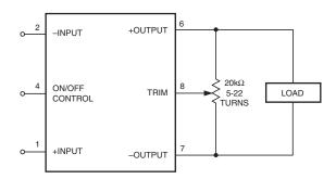
Figure 5. Trim Connections Using A Trimpot
