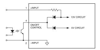
Figure 2. Driving the Positive Polarity On/Off Control Pin
