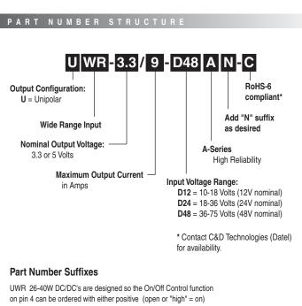
UWR 26-40W DC/DC's are designed so the On/Off Control functior on pin 4 can be ordered with either positive (open or "high" = on) or negative (open = off, pull low = on) polarity. The standard part number with no suffix denotes positive polarity. Add an "N" suffix to select negative polarity.
