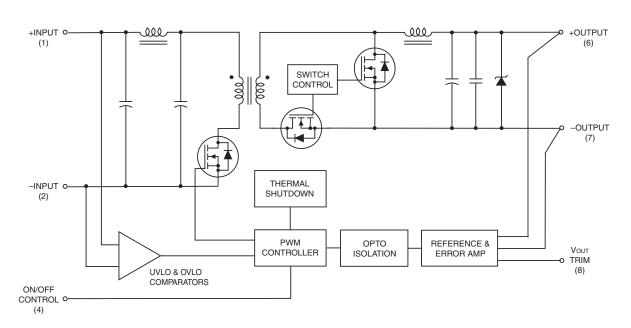
Figure 1. Simplified Schematic
