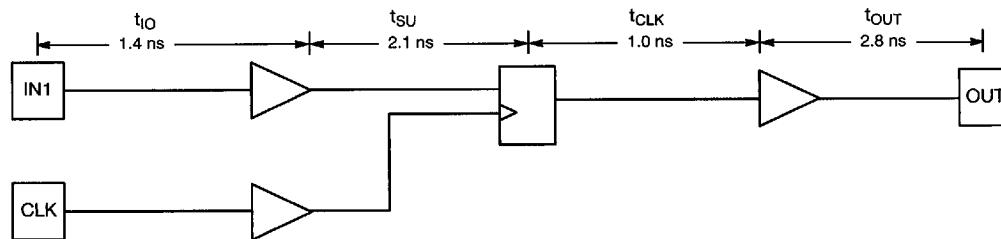
INPUT DELAY + REG SET-UP + CLOCK TO Q DELAY + OUTPUT DELAY = 7.3 ns
