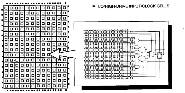
68, 84(85), or 100 PINS, INCLUDING 68 I/O CELLS, 6 INPUT HIGH-DRIVE CELLS, 2 INPUT/CLK (HIGH-DRIVE) CELLS
