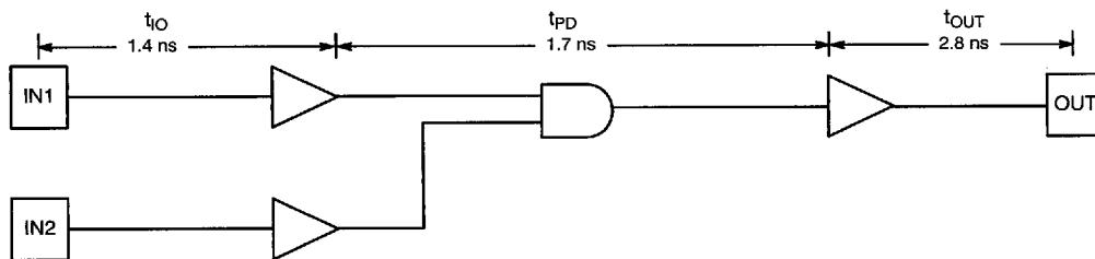
INPUT DELAY + COMBINATORIAL DELAY + OUTPUT DELAY = 5.9 ns
