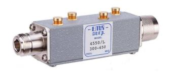
EMR Low-Pass Filters pass signals with a frequency lower than a certain cutoff frequency and attenuate signals with frequencies higher than the cutoff frequency, eliminating harmonics and IM products above the fundamental transmitter fundamental frequency. These filters come standard with N-Female to N-Male connectors. Other RF connector options available upon request.
