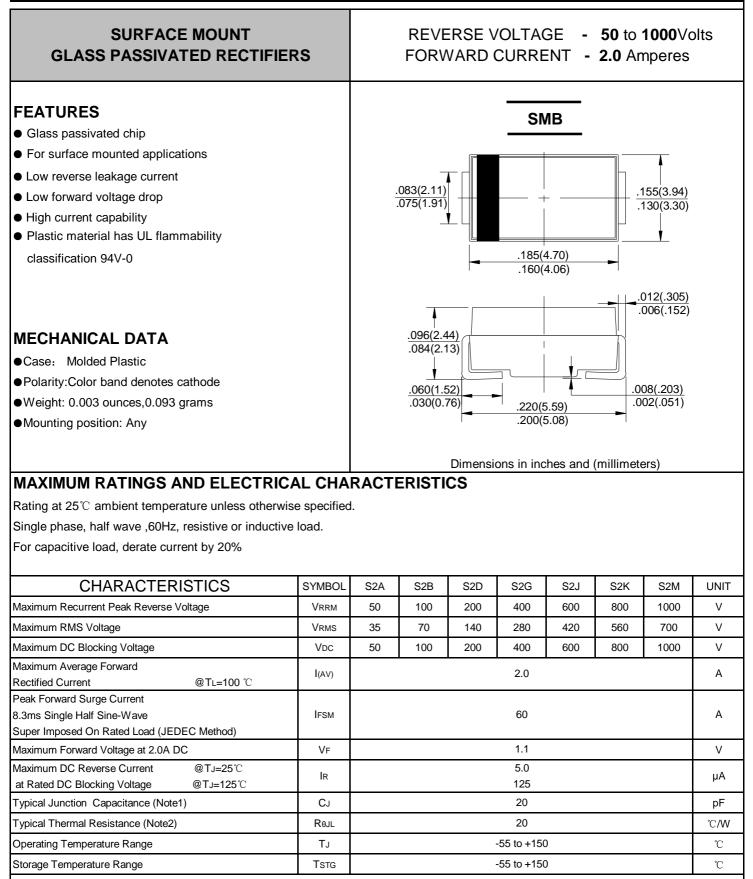
NOTES:1.Measured at 1.0 MHz and applied reverse voltage of 4.0V DC.
