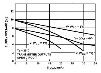
FIGURE 10. V+, V- OUTPUT VOLTAGE vs LOAD
