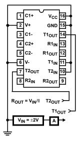
FIGURE 2. POWER-OFF SOURCE RESISTANCE CONFIGURATION
