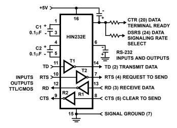
FIGURE 7. SIMPLE DUPLEX RS-232 PORT WITH CTS/RTS **HANDSHAKING**
