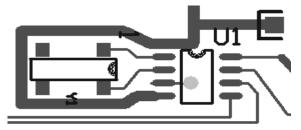
FIGURE 19. SUGGESTED LAYOUT FOR ISL1208 AND CRYSTAL
