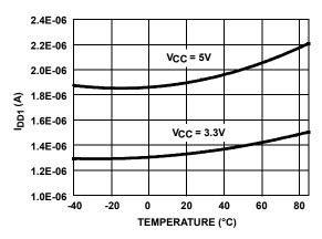
FIGURE 3. I<sub>DD1</sub> vs TEMPERATURE
