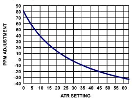
FIGURE 18. ATR SETTING vs OSCILLATOR FREQUENCY ADJUSTMENT
