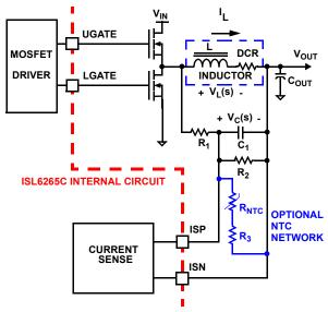
FIGURE 10. DCR SENSING COMPONENTS
