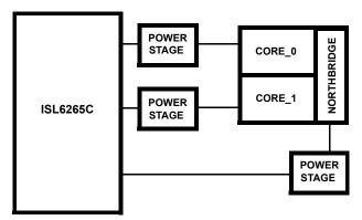
FIGURE 1. SIMPLIFIED SYSTEM DIAGRAM
