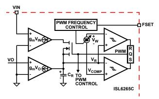
FIGURE 6. MODULATOR CIRCUITRY
