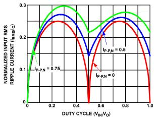
FIGURE 13. NORMALIZED RMS INPUT CURRENT FOR 2-PHASE CONVERTER
