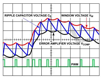
FIGURE 7. MODULATOR WAVEFORMS DURING LOAD TRANSIENT
