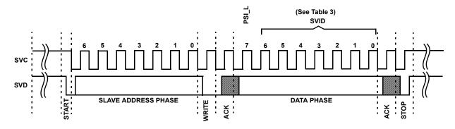
FIGURE 9. SEND BYTE EXAMPLE
