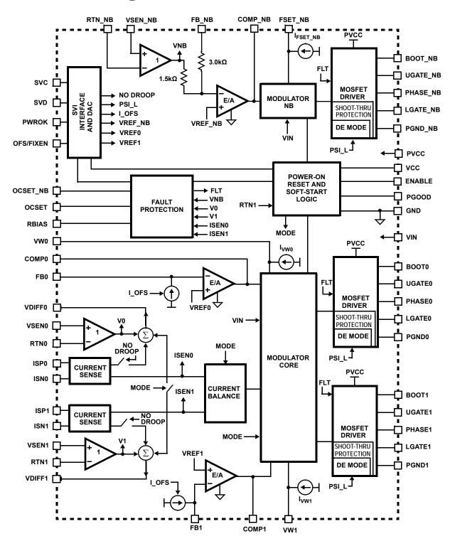
FIGURE 2. SIMPLIFIED FUNCTIONAL BLOCK DIAGRAM OF ISL6265C
