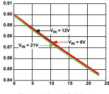
Figure 1.  $V_{CORE}/VR$  A Load Line = 2.4m $\Omega$
