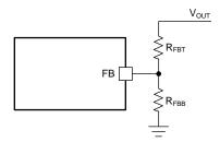
Figure 14. Output Voltage Setting
