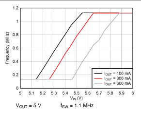
Figure 17. Frequency Foldback at TOFF MIN
