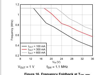
Figure 16. Frequency Foldback at Ton MIN
