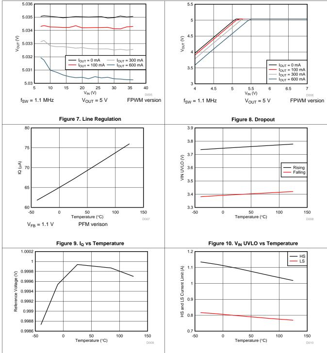
Figure 11. Reference Voltage vs Temperature
