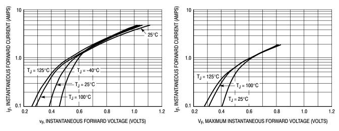
Figure 1. Typical Forward Voltage
