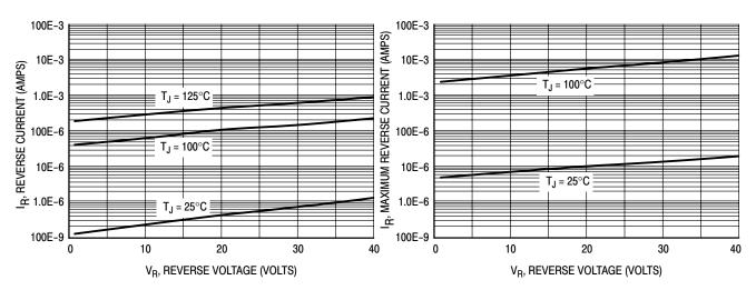
Figure 3. Typical Reverse Current
