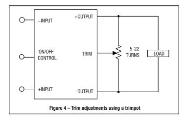
CAUTION: Be careful of external electrical noise. The Trim input is a senstive input to the converter's feedback control loop. Excessive electrical noise may cause instability or oscillation. Keep external connections short to the Trim input. Use shielding if needed.
