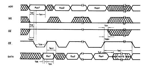
\*NOTE 1. I/O7 Outputs Dinn when the chip is read. I/Os is toggling between "1" and "0" when the chip is successively read
