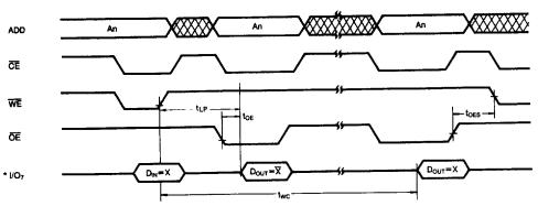
\* During the write cycle, I/O $_7$  will produce an inverted data of the last I/O $_7$  data, loaded into the EEPROM
