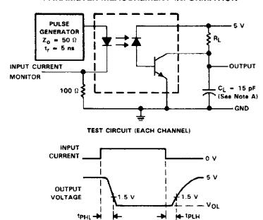
NOTE A:  $C_L$  includes probe and stray capacitance.
